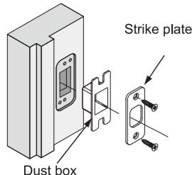
Use the strike plate as a template to drill the latch and screw holes and chisel out the mortise. The strike plate must fit flush with the surface of the door jamb.
