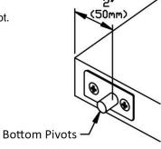
FASTEN BOTTOM PIVIT BRACKETS FLOOR BRACKET to floor 5/16"(8mm) from jamb face and centered under track. Remove floor bracket. Hang pivot door by inserting top pivots into top pivot brackets. Lock into place with locking lever. Tilt door slightly to allow bottom pivit brackets to slide under bottom pivots. Insert bottom pivots into hole of bottom pivit brackets. Reattach floor bracket.
