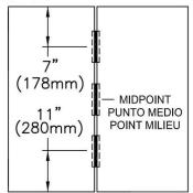
MARK a line 1/2" (13mm) from jamb side door edge along top of all doors (or on centerline). Mount Top Pivot on jamb door and Hanger Door Plate 1121 on other doors (see diagram). Bottom Pivot is located 5/8" (16mm) from edge of jamb door 2" (50mm) to center of Pivot. NOTE: Locking Latch must open toward rear of opening.
