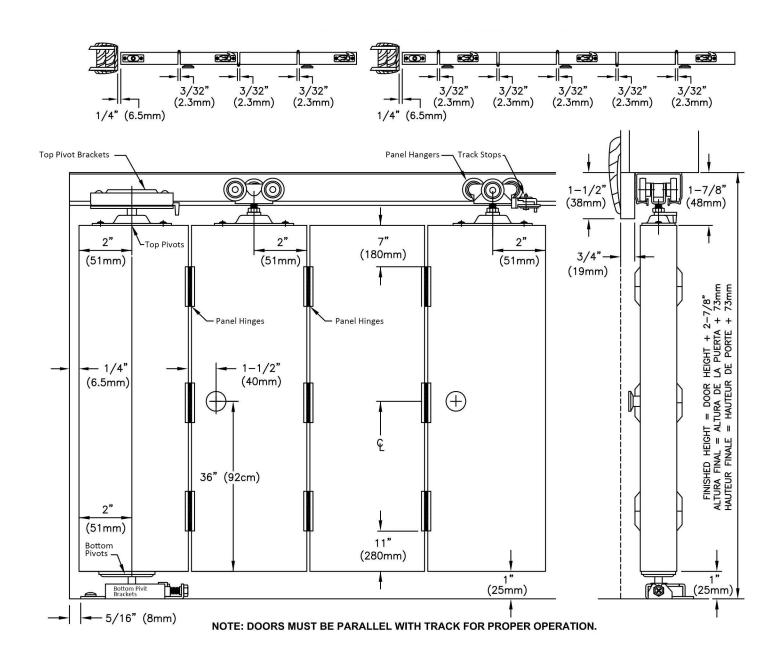
TRACK TO LENGTH. Insert parts in track and fasten to center of header with 1-1/4" (32mm) pan head screws.
